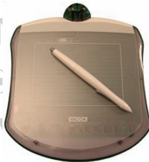
Figure 1.12 Drawing tablets such as this Wacom can be used instead of a mouse to draw images.
