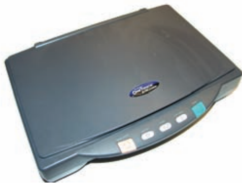
Figure 1.9 Scanners transfer printed images into digital images by using light technology.
