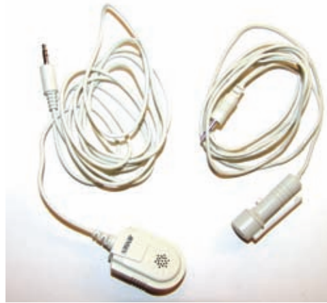
Figure 1.10 Small microphones such as these can be used to transfer voice to a computer.
