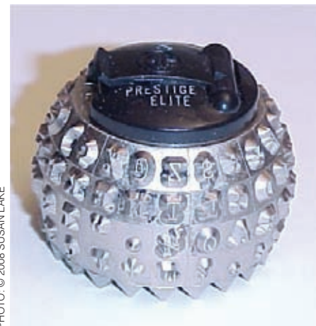
Figure 1.2 The design of the Selectric golf ball element provided options in font sizes and styles.
