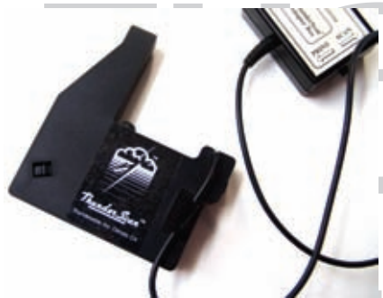
Figure 1.5 Thunderscan™ developed an early scanner that replaced the printer ribbon in an ImageWriter.
