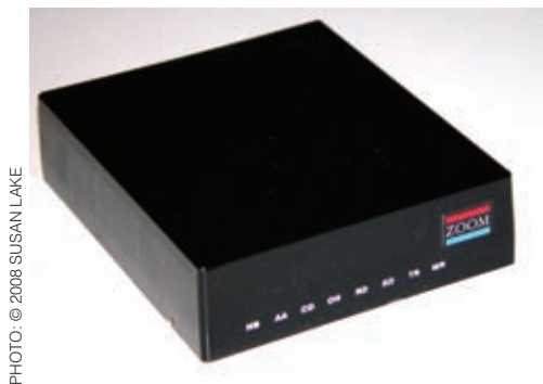
Figure 1.17 A modem allows one computer to talk with another, creating a network.
